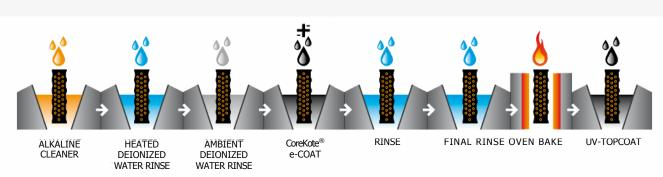
e-Coating is the process by which a metallic work piece (coil) is submerged in a paint / water bath where electricity is used to deposit paint onto it. CoreKote® e-Coat is a factory-applied corrosion-retardant coil coating which is applied in one of our four e-Coat facilities.
