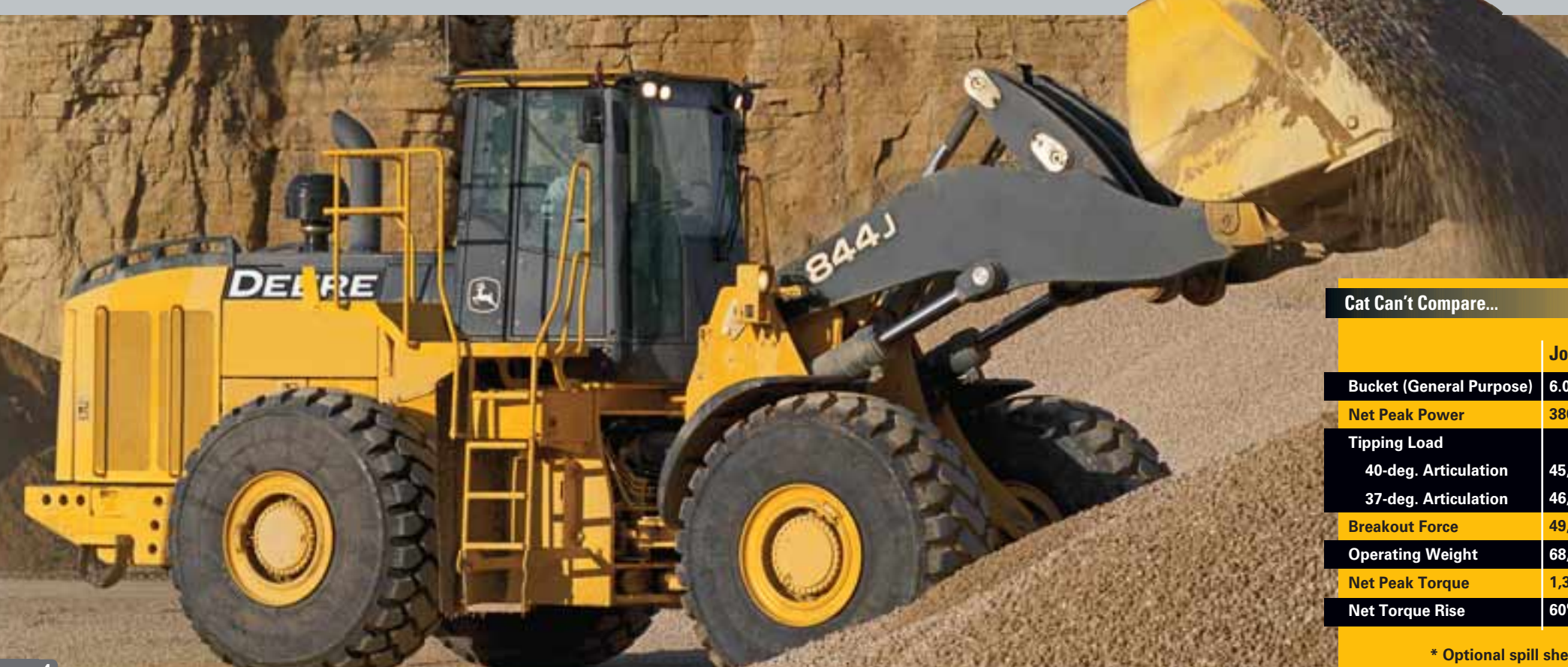
LOADRITE WEIGH SYSTEM: The 844J is Loadrite-Weigh-Management-System ready, so you can load each truck to its full legal payload for maximum productivity. The loader is pre-wired and pre-plumbed for fast installation, and includes a standard mounting pad for the Loadrite monitor.
